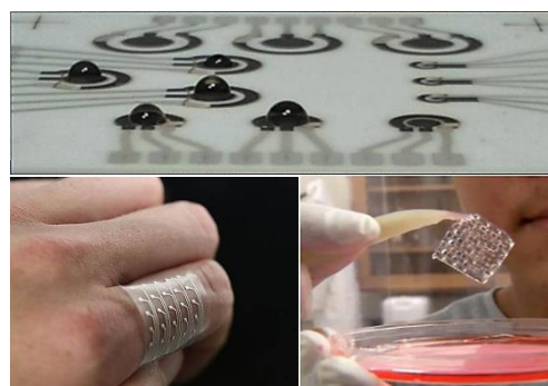
Fig. 1. Different types of ion-selective sensors printed in AJP and wearable sensors.
