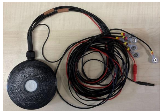
Figure 1. FitFES device: two electromyographic channels and one stimulation channel.
