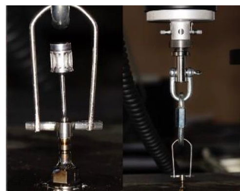
Fig. 1: traction test using Instron machine to test traction resistance of Orbit® intermediate connection
